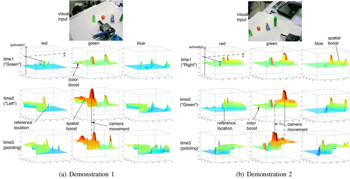
Fig. 2. Snapshots of activity of the color-space dynamic fields at decisive time-points in the dynamics during the two robotic demonstrations (see text for details).
