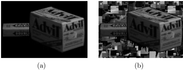
Figure 16: Input images of a partially occluded object. (a) A segmented and (b) an unsegmented input image of a partially occluded object. In this example, the occluding object covers about 50% of the occluded object.
