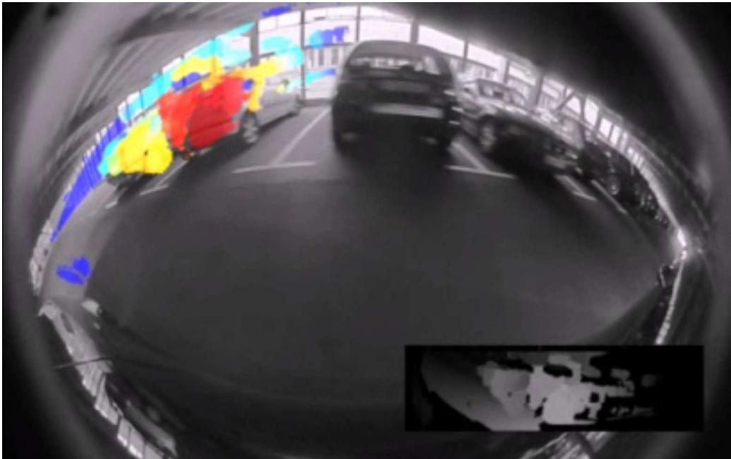
Figure 9. Video 2: The color-coded disparity estimation in a sequence seen from the right side mirror camera. The vehicle performs a short drive through a roofed parking deck. http://dx.doi.org/doi.number.goes.here
