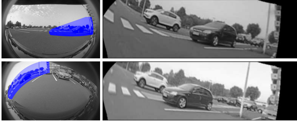
Figure 5. The input and rectified images from the front (top) and right (bottom) camera of the presented topview setup. The overlapping field of view is indicated.
